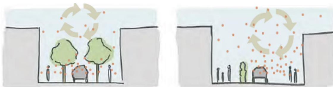
Figure 3.5: Street canyon where air at street level is more polluted than the air above
